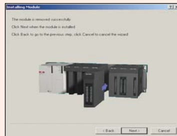
Module exchange wizard It supports safe module exchange during 'RUN' mode.
