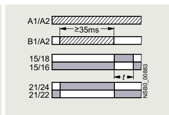
F•¹) 3RP2005-.B Passing break contact with control signal and instantaneous contact
