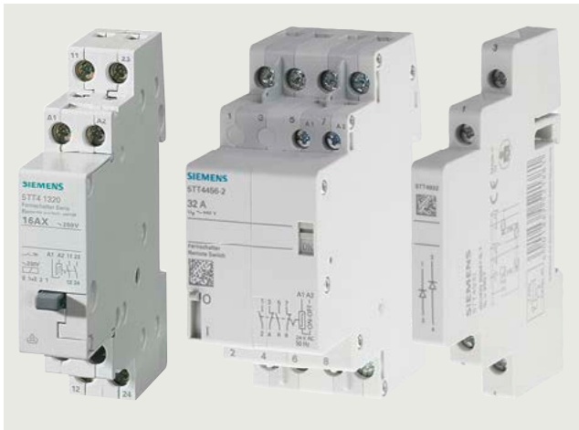
5TT4101-0 remote control switch for AC applications, up to 16 A, 2 NO contacts (left) 5TT44 remote control switch for AC applications, 2 CO contacts (center) 5TT4930 auxiliary switch for 5TT44 remote control switches, 1 NO + 1 NC (right)
