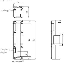
01) When removing the end cap, there is the lamp output terminal (top) or the power supply terminal (bottom).02) When removing the front cover, there is the setting switch (on the emitter and the receiver) or the PC communication port (on the receiver).
