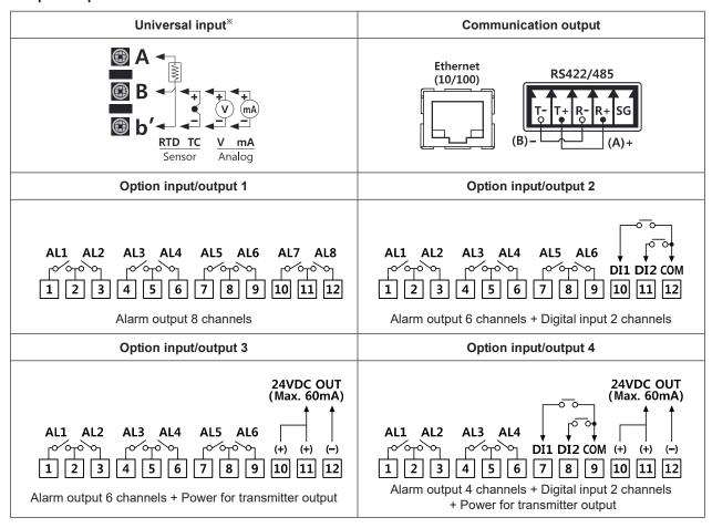
$\ensuremath{\mathbb{X}}$  In case of current input, connect  $250\Omega$  resistance at external part.
