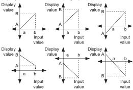
Display scale function is able to change display value for max./min. measured input by setting high-limit scale and low-limit scale.
