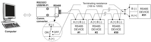
XIt is recommended to use Autonics communication converter; SCM-WF48 (Wi-Fi to RS485·USB wireless communication converter, sold separately), SCM-US48I (USB to RS485 converter, sold separately), SCM-38I (RS232C to RS485 converter, sold separately). Please use twisted pair wire, which is suitable for RS485 communication, for SCM-WF48 and SCM-US48I.
