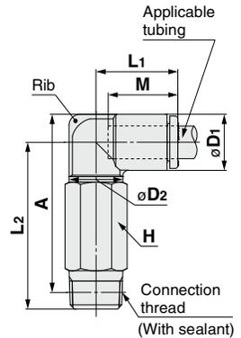
□: A (Brass), N (Brass + Electroless nickel plating) \*1 Reference dimensions after installation of R thread
