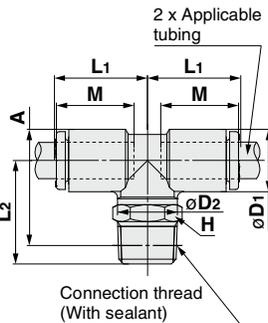
□: A (Brass), N (Brass + Electroless nickel plating) \*1 Reference dimensions after installation of R thread
