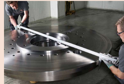
Radiused jaws for accurate ID measurement
